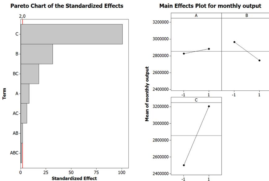
Figure 6 - Pareto chart and Main effects plot for monthly parts production
