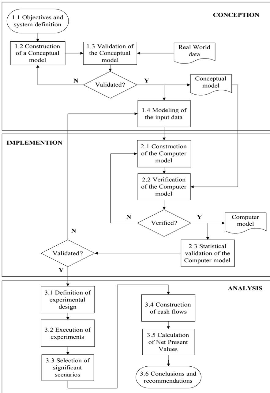
Figure 1 - The sequence of steps for this simulation study
