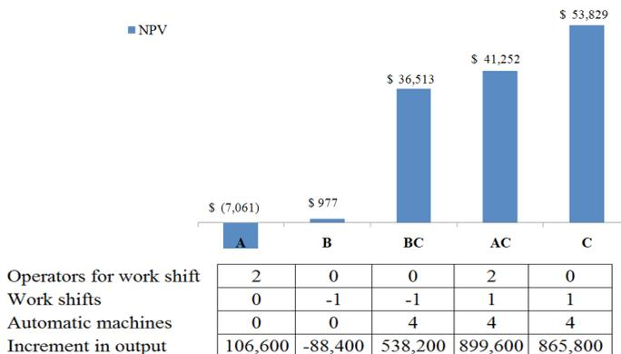
Figure 9 - Classifications of the scenarios for the automotive manufacturing cell
