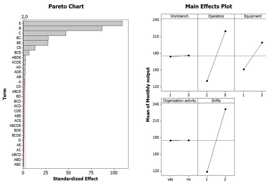
Figure 7 - Pareto Chart and main effects plot for monthly transponder B production
