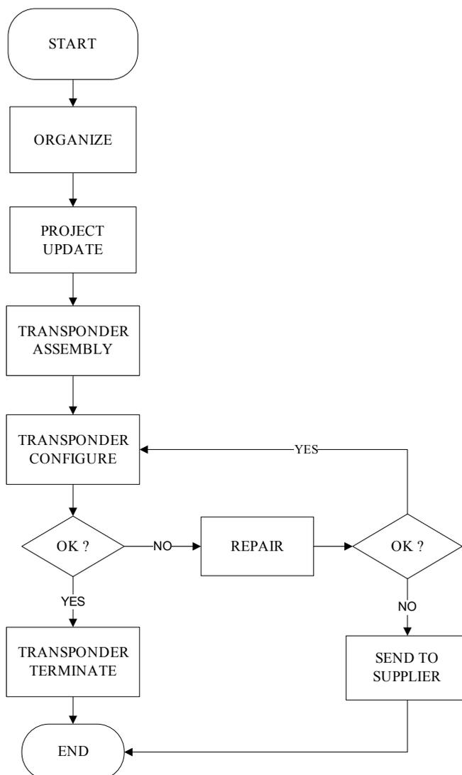
Figure 2 - Flow chart of the transponder A process, the simulation conceptual model
